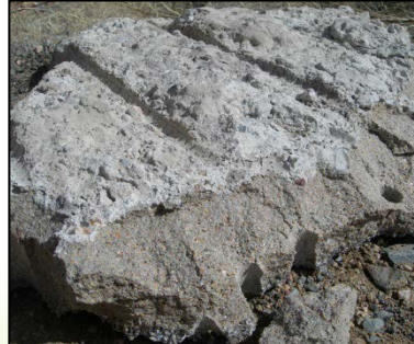
Thermal compatibility, unsound substrate
