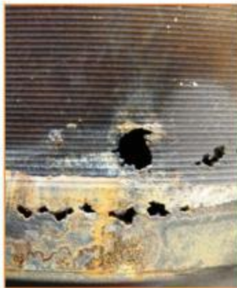
Coolant leaks by liner cavitation
