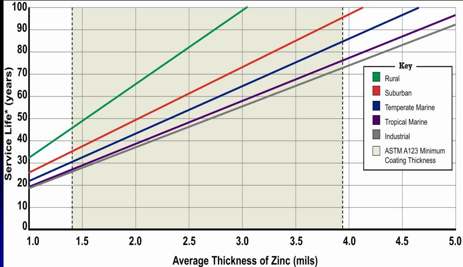
\*Service life is defined as the time to 5% rusting of the steel surface. 1 mil = 25.4µm = 0.56oz/ft<sup>2</sup>
