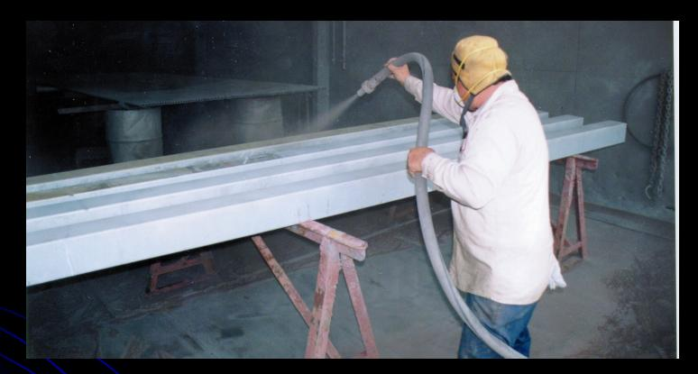
Standard Practice for Preparation of Zinc (Hot-Dip) Galvanized Coated Iron & Steel Product & Hardware Surfaces for Painting
