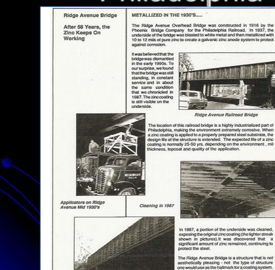
The location of this railroad bridge is a highly industrialized part of Philadelphia, making the environment extremely corrosive. When a zinc coating is applied to a properly prepared steel substrate, the design life of the structure is extended. The expected life of a zinc coating is normally 25-50 yrs. depending on the environment , mil
