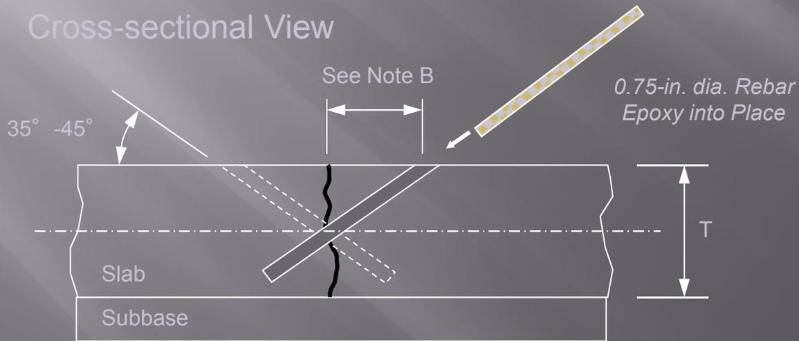
**Note A:** Distance between holes is 24 in. for heavy traffic; 36 in. for light traffic
