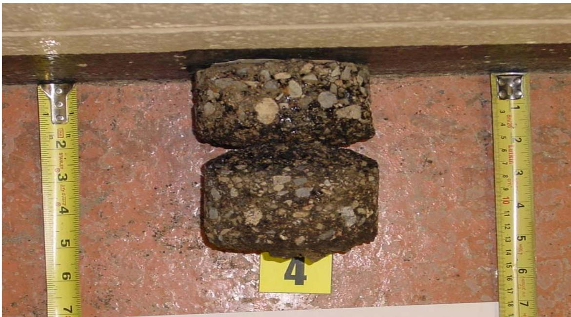
3 Years after Construction: Delaminated at 2.3 in. with Medium to Heavy Stripping
