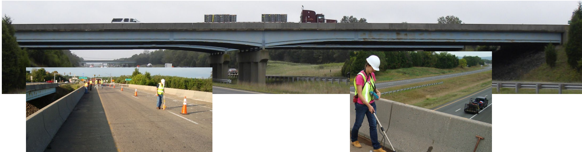
Half-Cell Potential Survey 2009
