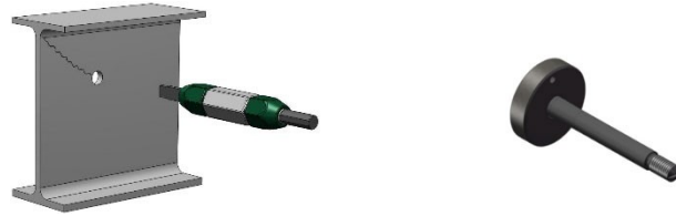
Hole quality and mandrel wear check
