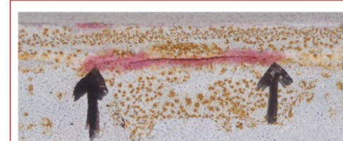
Before: Typical Weld Line Crack
