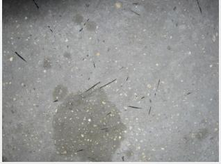
Square patch: a few fibers are visible on the surface, probably due to abrasion.
