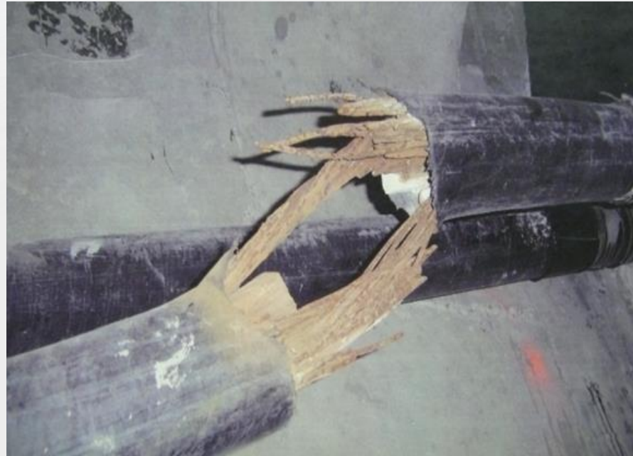
Soft Grout or Voided Duct Resonant Frequency = 7,000 Hz
