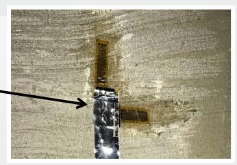
Strain gauge sensor:
