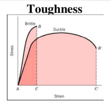
Toughness = the ability to absorb energy up to fracture
