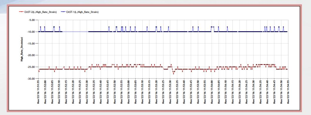
Front axles on top of culvert Strain change is negligible Rear axles on top of culvert Strain change, negligible
