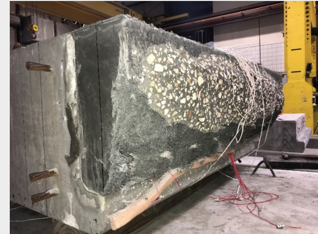
Debonding between UHPC and precast concrete
