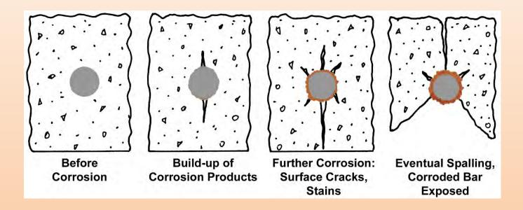
Corrosive elements - water, air, chlorides,  $CO_2$  - diffuse through the concrete matrix to reach rebar
