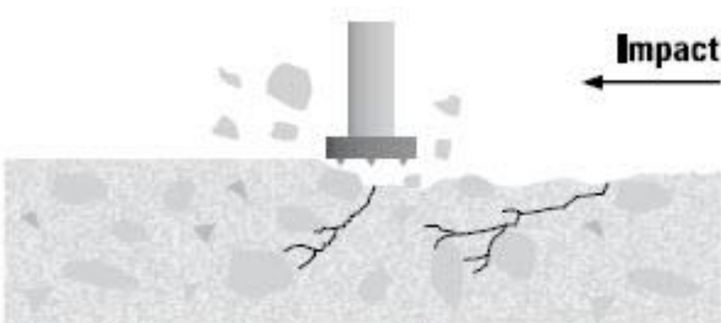
Fig. 4.3: Scarifying, scabbling, rotomilling, needle scaling
