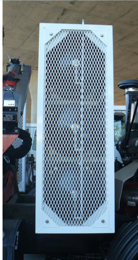
UV Damage –supplier installed solid panel
