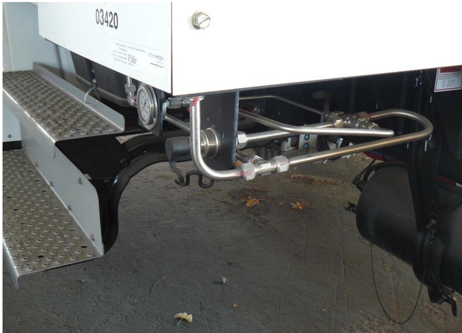
Potential Road Debris Damage -supplier corrected later
