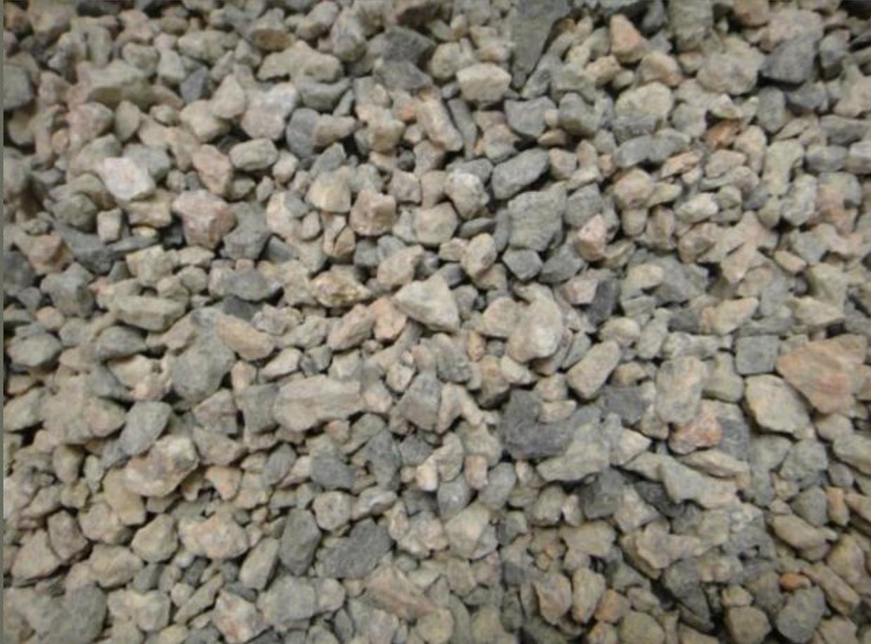
**Mill Creek Aggregate (1/4-in chips)
