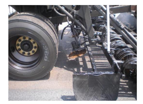
Spring-loaded tines set hydraulically at prescribed depth will drag over existing structures to avoid damage
