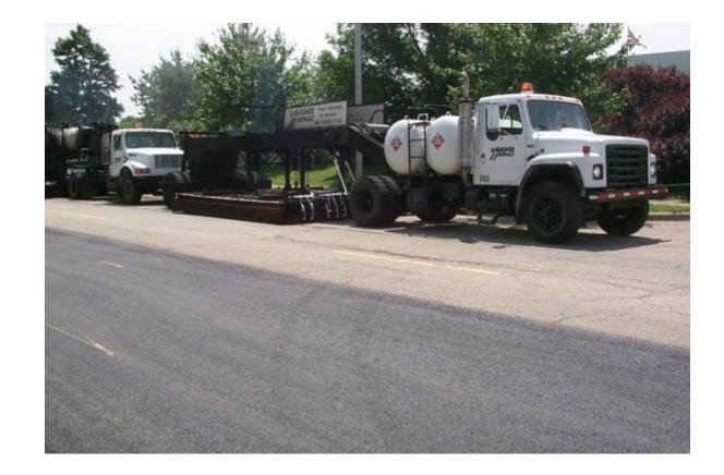
2<sup>nd</sup> Heater takes pavement temp to 280 – 300 degrees
