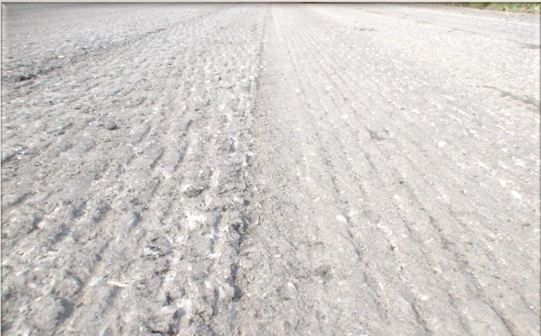
8 mm Triple Wrap Fine Drum (300 Bits) Vs. 22.5mm-15/16" Quad Wrap Standard Drum (200 Bits) Both Milled at 85' /Minute
