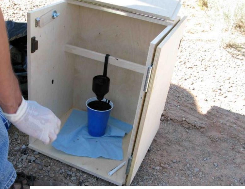
20 to 70 seconds at 85 to 150F for a 6 mm orifice or 10 to 60 seconds at 85 to 140F for a 7.5 mm orifice
