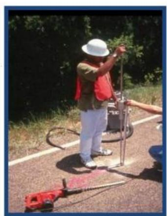
Measures both layer stiffness (from penetration rate) and layer thickness (change in penetration rate)
