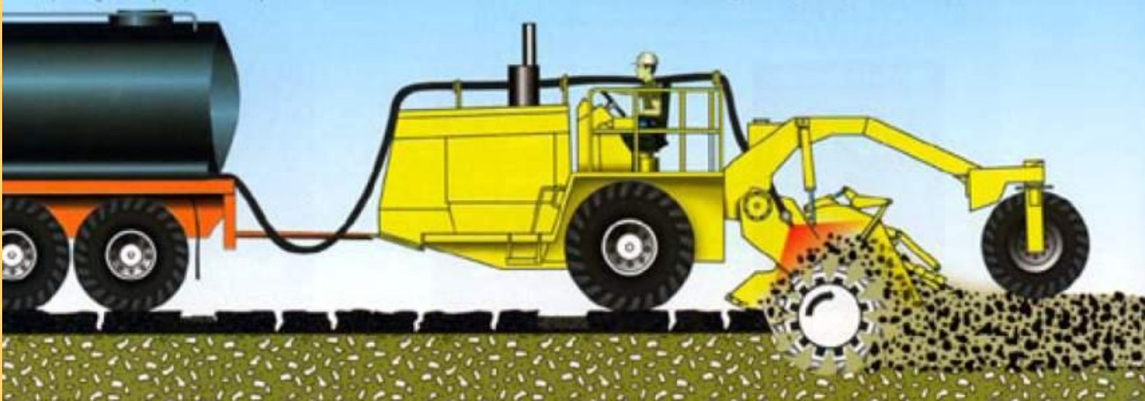
FDR'S PULVERIZATION AND MIXING PROCESS
